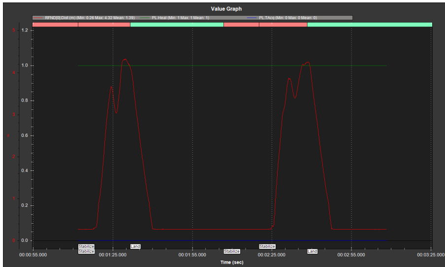
Figure 28: Flight log showing UAV height above ground (red), IR-lock camera health (green) and IR beacon detection status (blue).
